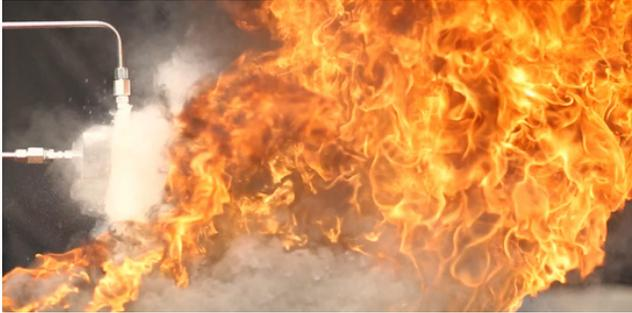
Dry chemical fire suppression systems provide the fastest fire knockdown and greatest total coverage, making them the industry standard for heavy equipment applications. Dry chemical systems provide fire protection against Class A (debris), Class B (fuel), and Class C (electrical) fires. This system is effective by flooding a volume of space, such as a vehicle engine compartment, with a fire fighting agent to suffocate the flame.
