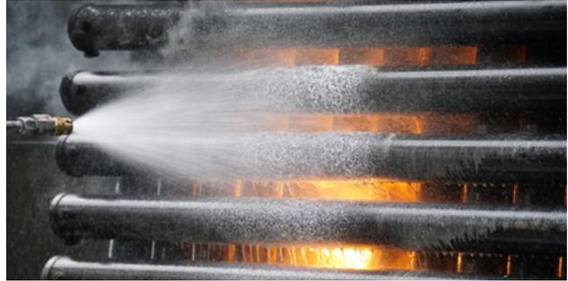
Liquid agent fire suppression systems provide exceptional cooling abilities to suppress Class A (debris) and Class B (fuel) fires. The liquid agent works by cooling hot surfaces, separating fuel hydrocarbon molecules to prevent fire reignition and form a layer of foam to suffocate flames. Liquid systems are especially designed to protect high risk vehicle components, such as turbochargers, exhaust components, and Tier 4 aftertreatment components.
